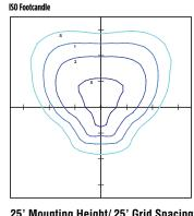
25' Mounting Height/ 25' Grid Spacing ■2 FC ■ 1 FC ■ 0.5 FC
