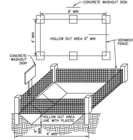
THE USE OF PORTABLE CONCRETE WASHOUT UNITS IS APPROVED (AND ENCOURAGED) FOR ALL CONSTRUCTION. THE EXACT LOCATION OF CONCRETE WASHOUT(S) MAY BE FIELD LOCATED BY THE ON-SITE PROJECT ENGINEER/CONTACT.
