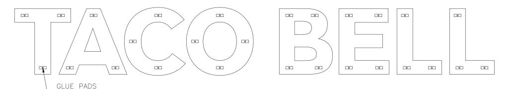
AS INSTALLATIONS WILL VARY GREATLY FROM LOCATION TO LOCATION, IT IS IMPOSSIBLE TO PROVIDE SPECIFIC INSTALLATION INFORMATION. TYPICAL INSTALLATION WILL INCLUDE A TOTAL OF (27) 5/16" AND (0) 7/8" PENETRATIONS IN THE FASCIA, UTILIZING 1/4"X2.5" (SIZE) STAINLESS THREADED RODS (PROVIDED).
