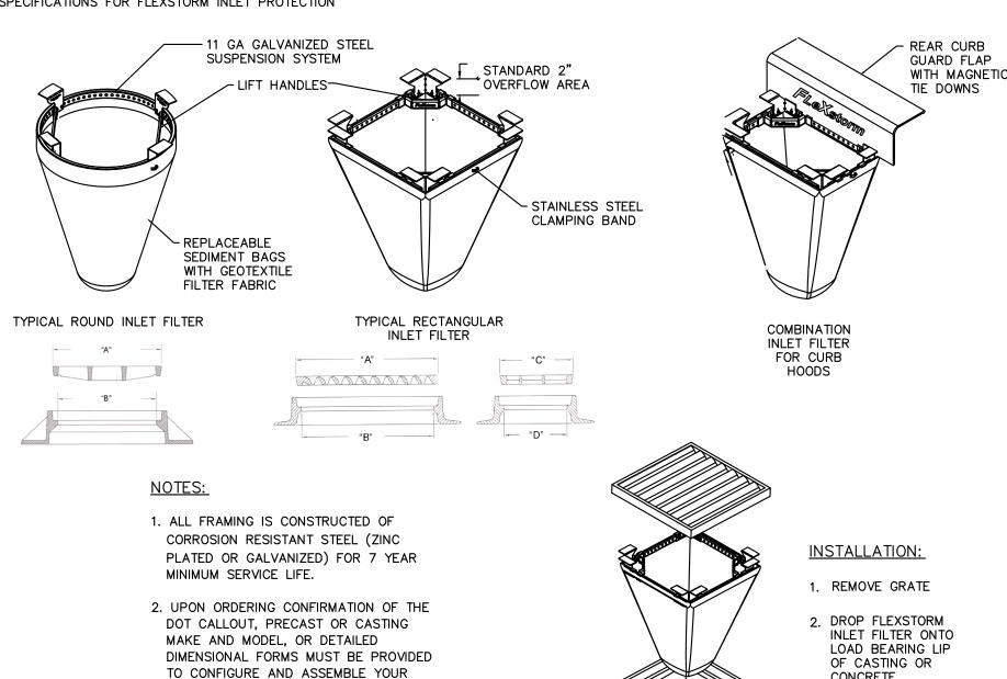
WWW.INLETFILTERS.COM FLEXSTORM TEMPORARY INLET PROTECTION DETAIL
