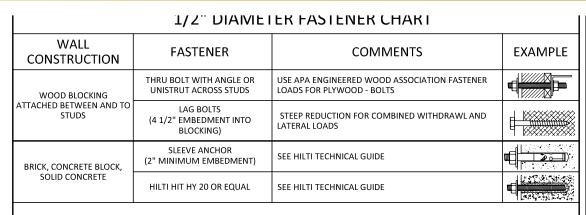
NOTE: ALL FASTENERS TO BE THRU BOLTS IF POSSIBLE, USE ALTERNATE FASTENERS PER WALL TYPE SHOWN ABOVE IF THRU BOLTING IS NOT POSSIBLE. ALL FASTENERS ARE TO BE CHOSEN AND PLACED IN ACCORDANCE WITH THE MANUFACTURER'S INSTALLATION INSTRUCTIONS.
